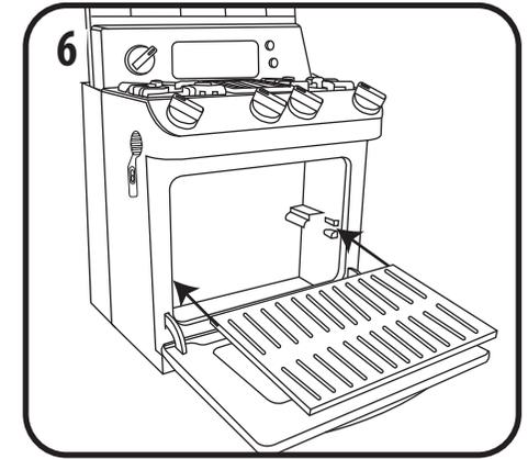
6 To insert the shelf, slide the sides of the shelf between the brackets in the oven.
