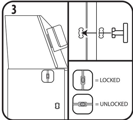
3 Insert a screw on each side of the top panel and turn the screw to lock in place. The screw should enter both openings.
