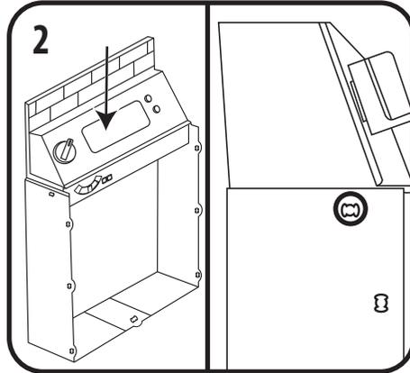
2 Insert the top panel on top of the back wall of the oven. The openings on each side should align.
