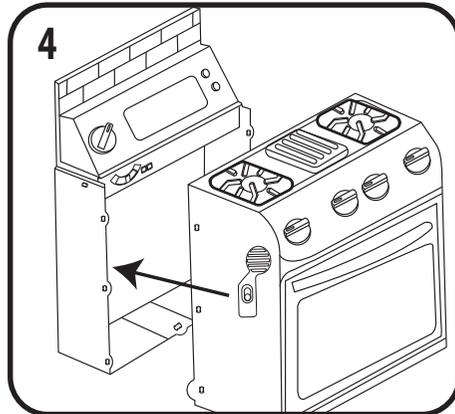
4 Slide the front of the oven into the back wall, making sure the openings on the sides and the one on the bottom align.
