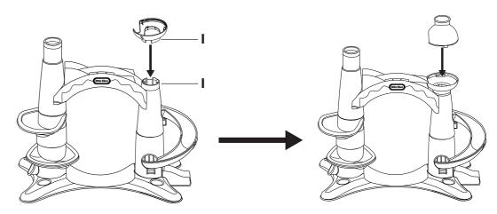
Attach the funnel (6) to the top of left tower, while lining up to the guides located on the top end of the tower and bottom of the funnel itself.
