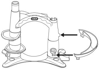
Connect the dome dish (9) to the top of the right tower, then attach the dome (10) to the top of the dish. Note: When both pieces are connected properly they will create a circular opening.
