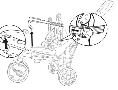
4. Fold seat down FIRST, then fold handlebars.
