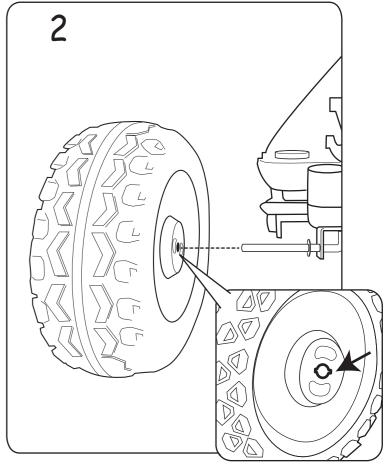
IMPORTANT NOTE: Spacers must remain in the axel openings on all four tires prior to installation.
