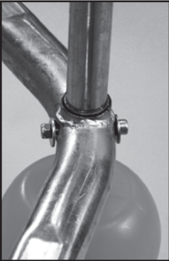
Insert bold (L) through the arc washer (O) then through the front opening in straight frame tube. Secure back with an arc washer (O), a spring washer (P) and cap nut (N). Tighten bolt assembly using the wrench (Q) to hold the cap nut in place while tightening bolt with the screwdriver (W).
