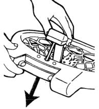
I have found that before putting the score bar on the rim applying some soapy water to the rim and pin help lubricate the plastic. The pin moves easily through the rim without having to enlarge the hole in the rim.
